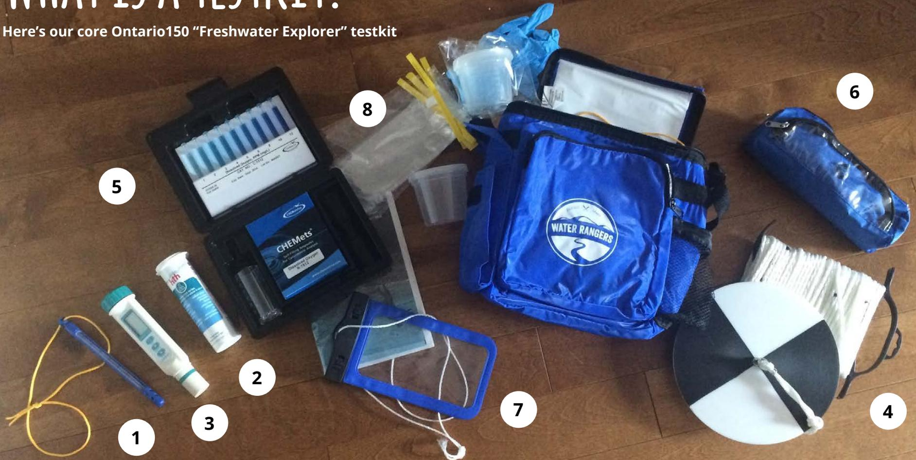
**1 Thermometer:** Air temperature, Water temperature \*
